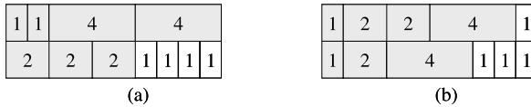
Fig. 4 (a) An optimal schedule. The bully jobs (in grey) are not scheduled according to SPT, \sum C_j = 65 . (b) The best schedule under the constraint that bully jobs obey SPT, \sum C_j = 66
