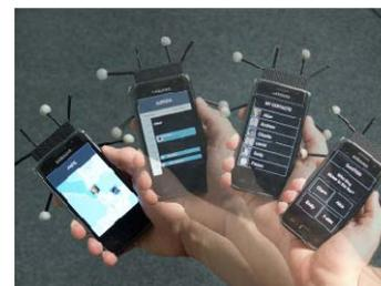
**Figure 3: mSpaces: spatially-aware mobile device. Different workspaces appear depending on the device’s position.**
